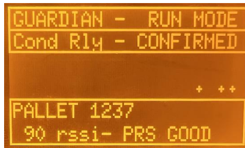
Figure 16: Run Mode Screen Simple System (Pressure Good)
