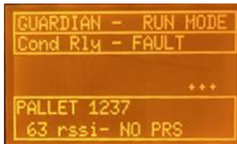
Figure 17: Condition Relay Status (No Pressure)
